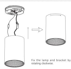
Connect the safety rope, and plug the earth wire connector, then plug the male and female connector.
