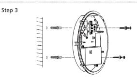
Fix the back housing on the wall or ceiling by screws.
