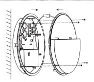
Connect the DC plug( if with Emergency , connect the plugs between the battery and driver), put back the cover to the back plate and fix it by screws
